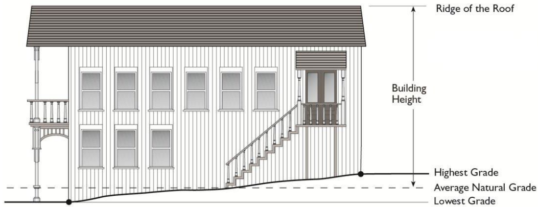
FIGURE 11.03.050(A): MEASURING BUILDING HEIGHT
